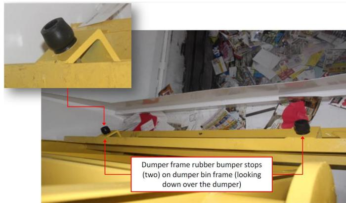
Figure 9. Frame Rubber Stops
