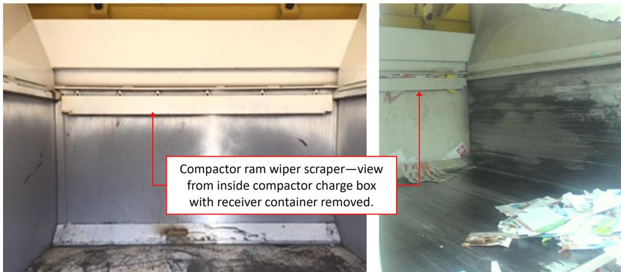
**Figure 36. Compactor Ram Wiper Scraper**
