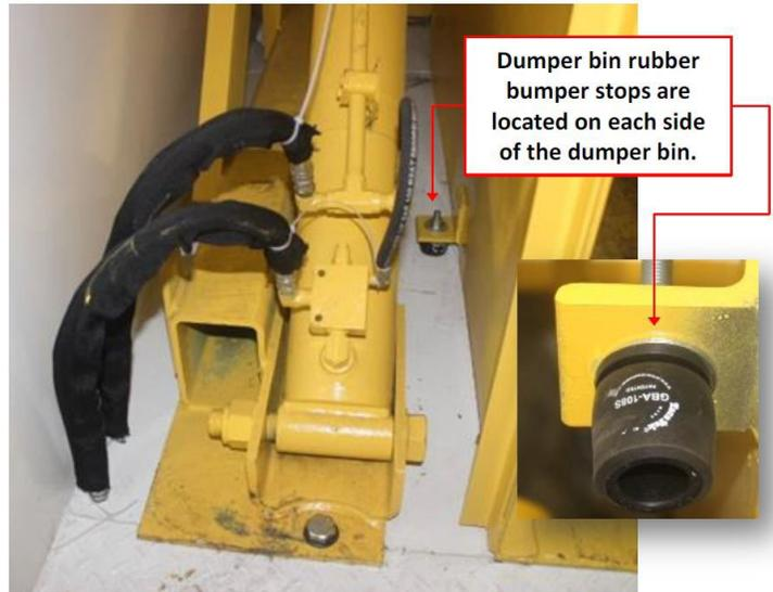
**Figure 8. Rubber Bumper Stops**
