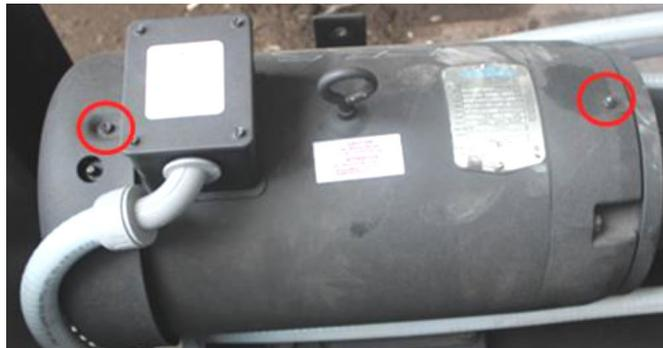
Figure 17. Motor Grease Fittings
