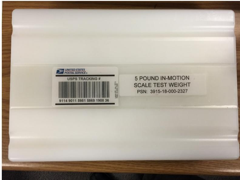
**Figure 1. 5-Pound In-Motion Scale Test Weight**
