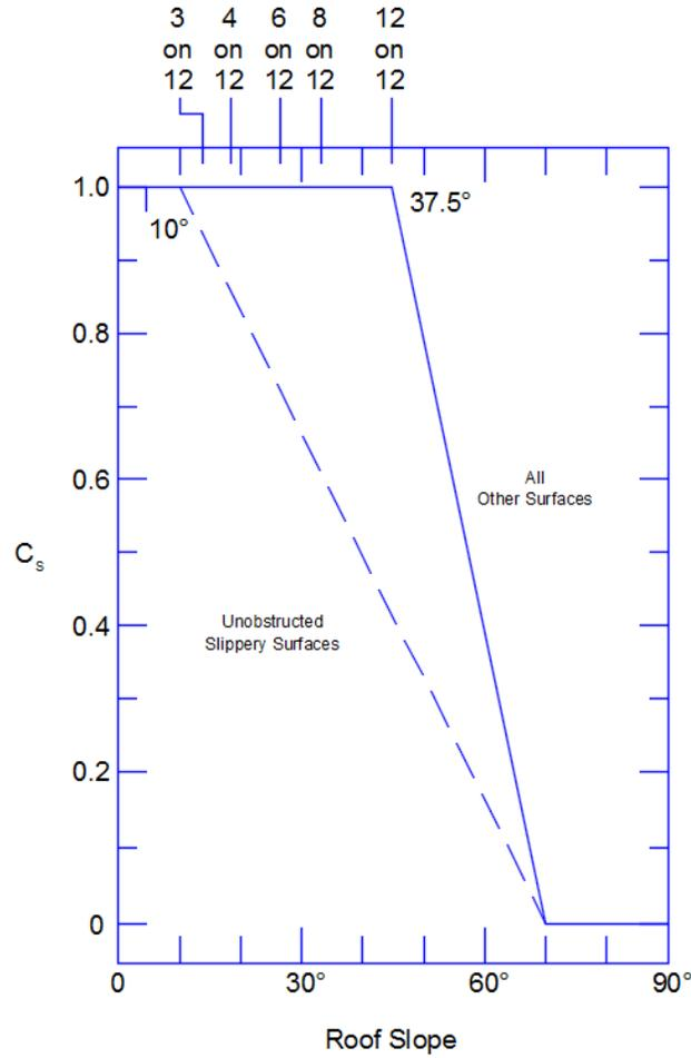
**Figure 4. Roof Slope for Cold Roofs with Thermal Factor (C<sub>i</sub>) = 1.1**
