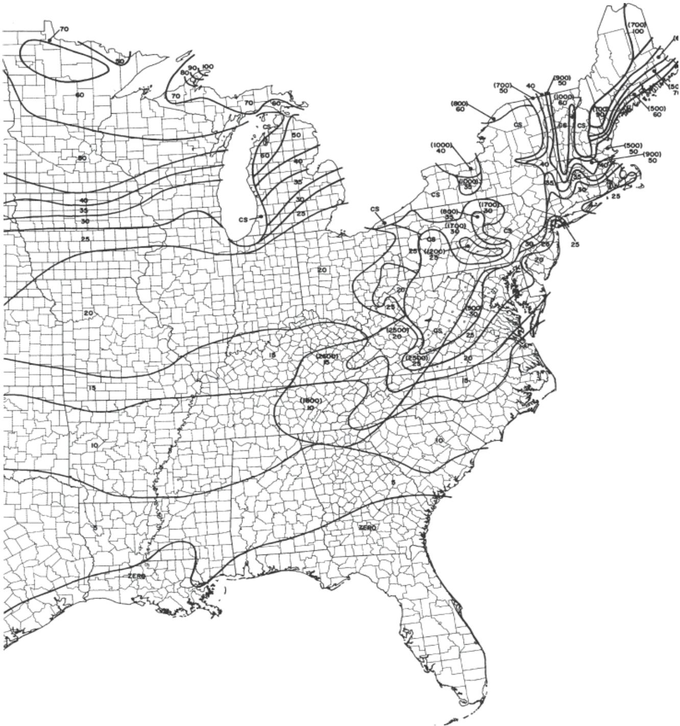
Figure 2. Ground Snow Loads ( $p_g$ ) in  $\text{lb}/\text{ft}^2$  for Eastern Half of USA
