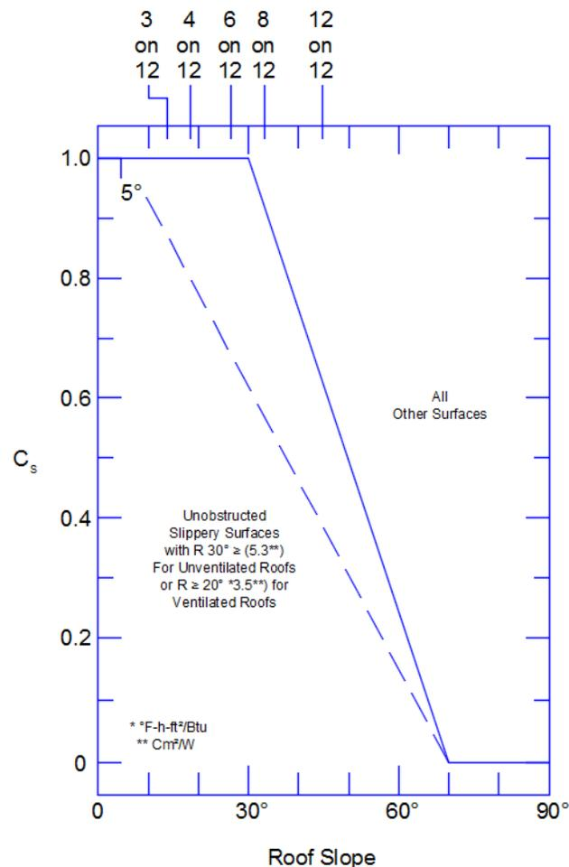
**Figure 3. Roof Slope for Warm Roofs with Thermal Factor ( $C_t$ )  $\leq 1.0$**
