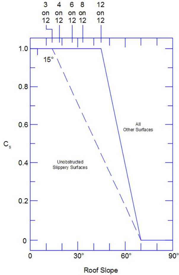
**Figure 5. Roof Slope for Cold Roofs with Thermal Factor ( $C_t$ )  $\geq 1.2$**
