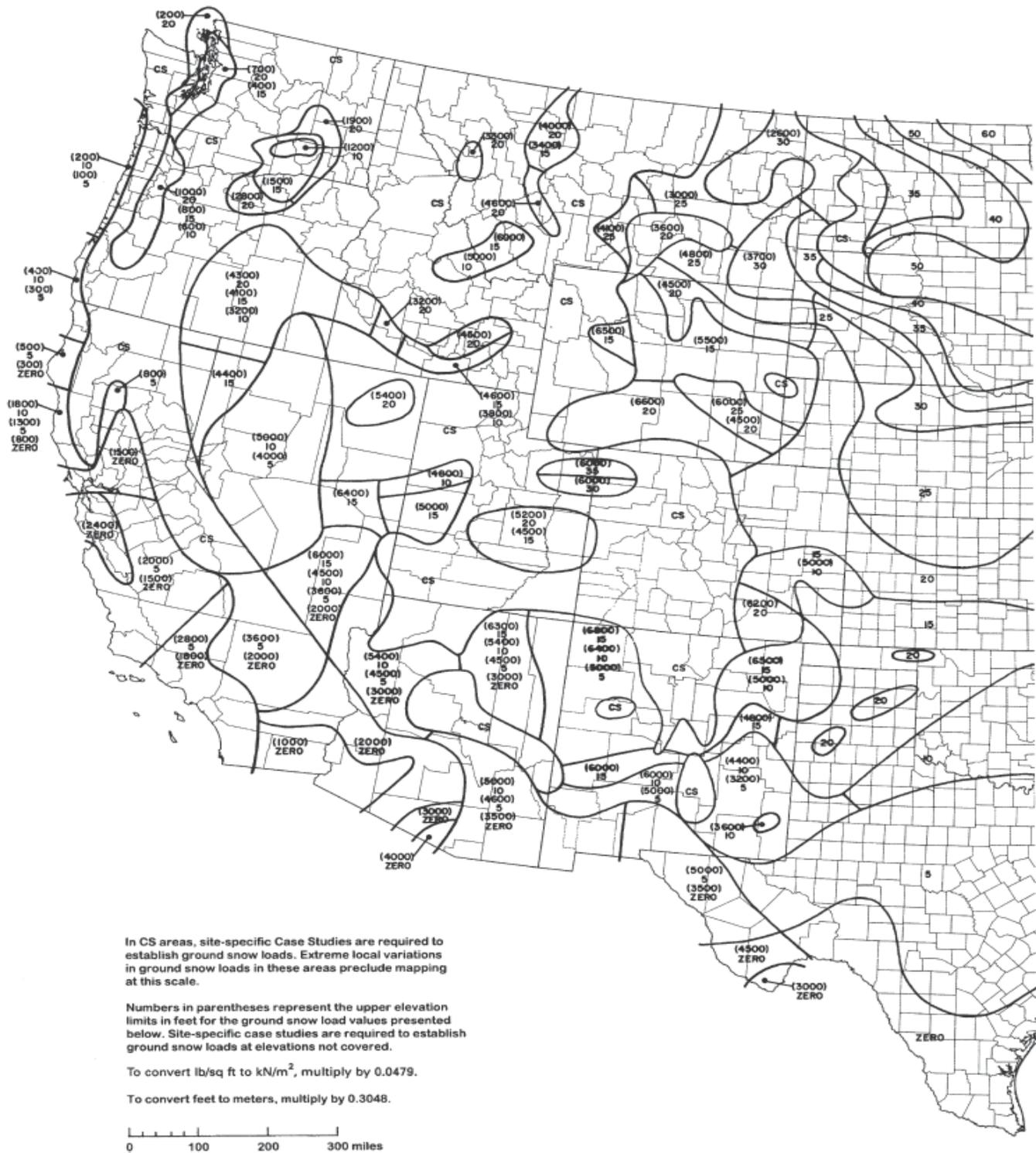
Figure 1. Ground Snow Loads ( $p_g$ ) in lb/ft<sup>2</sup> for Western Half of USA
