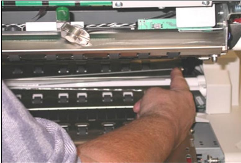
Figure 14. Removing/Replacing Glass Flat
