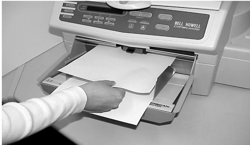
**Figure 9. Holding/Feeding Cleaning Sheet**
