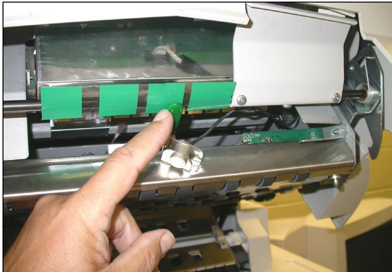
Figure 22. Inprinter Positioning Handle
