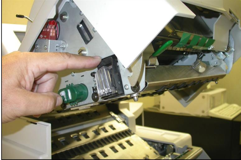
Figure 23. Imprinter Print Cartridge
